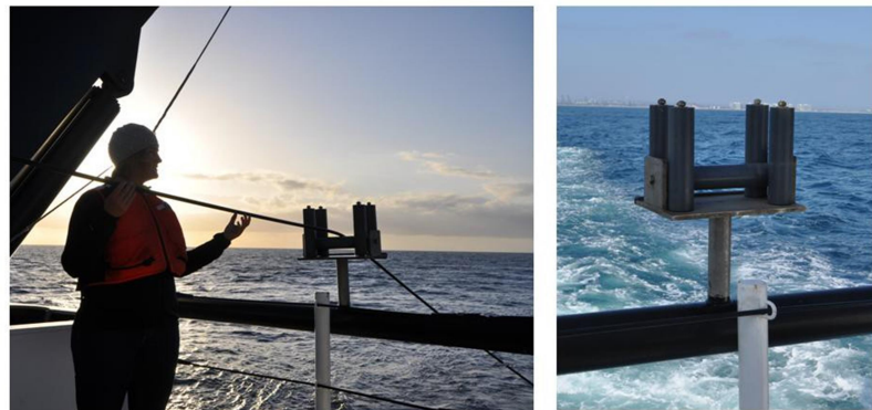
Figure 4. Roller to aid in deployment/retrieval of array from aft deck. Roller can be removed by lifting (requires 2 people).
