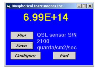
Using BSI's new operating software, the QSR-2100 logs and displays calibrated data in either Quanta or µEinsteins .
