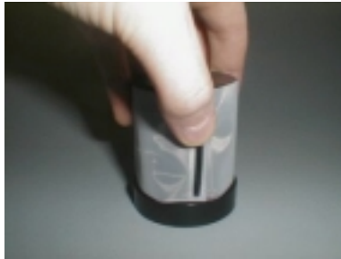
Figure F-4: Insert a plastic shim
