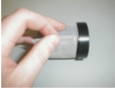
Figure F-3: Overlap the cloth over a groove
