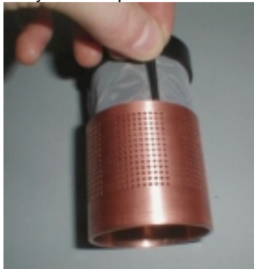
Figure F-5: Start positioning the copper screen
