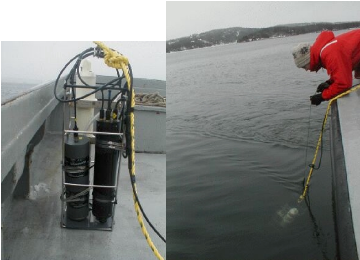
Figure C-3: CTD, ISUS, and Battery Pack
