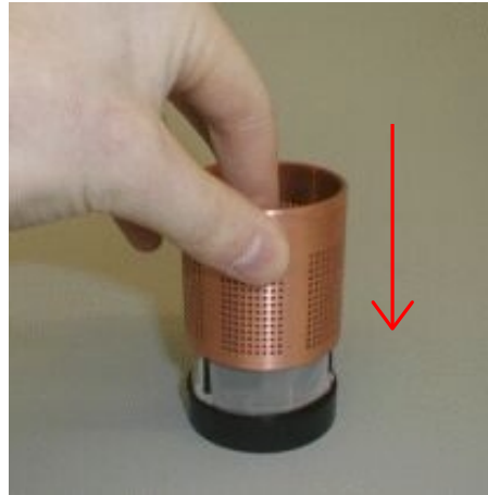
Figure F-6: Slide the copper screen in place
