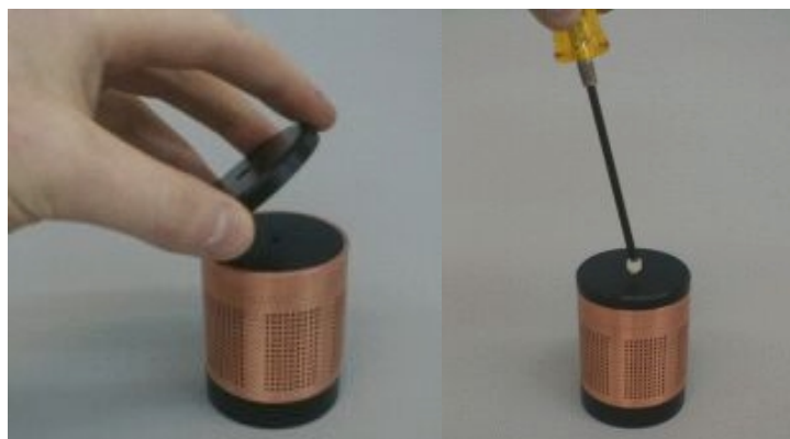
Figure F-7: Attach the end cap
