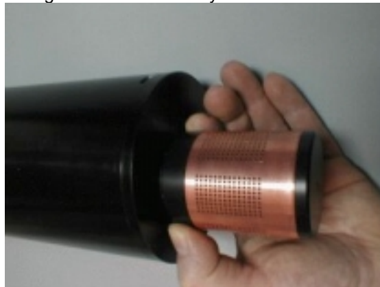
Figure F-9: Mounting the guard
