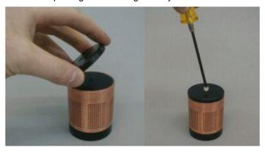
Figure F-7: Attach the end cap
