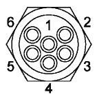
Figure A-7: MCBH6M Bulkhead, Male Face View
