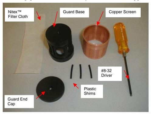
Figure F-1: Biofouling Guard Components
