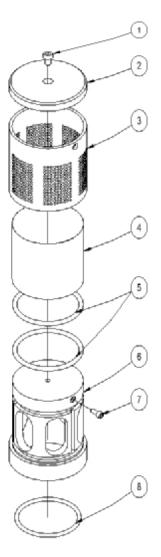
Figure F-2: Biofouling Guard Exploded Assembly
