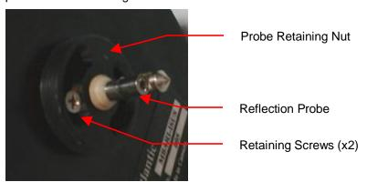
Figure A-12: Reflection Probe
