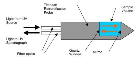
Figure A-3: Seawater Sample Illumination
