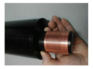
Figure F-9: Mounting the guard
