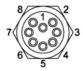
Figure A-9: MCBH8M Bulkhead, Male Face View
