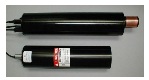
Figure A-1: The MBARI-ISUS with Rechargeable Battery Pack
