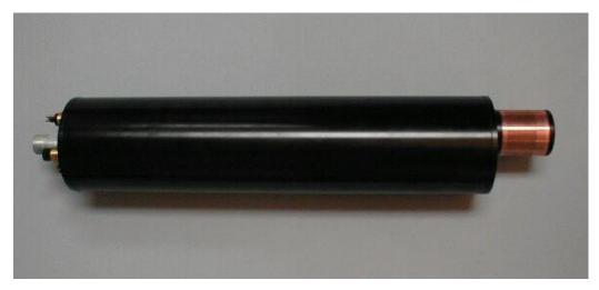
Figure F-10: The ISUS with Biofouling Guard
