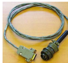
CDO Remote Out Interface test cable
