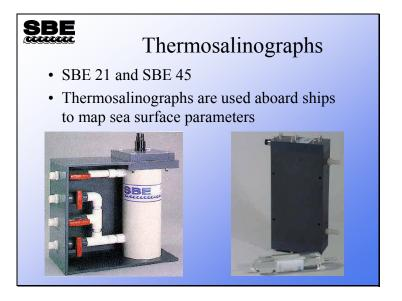
Thermosalinographs are used to collect information about the sea surface; typically in flow-through systems operating continuously throughout a cruise. They are included in the profiling section of the course because they are installed on many research vessels. Thermosalinographs are typically installed inside and near to the hull of a ship in order to make measurements on uncontaminated seawater. Optionally, you can plumb other types of sensors into the system for a wider range of measurements.
