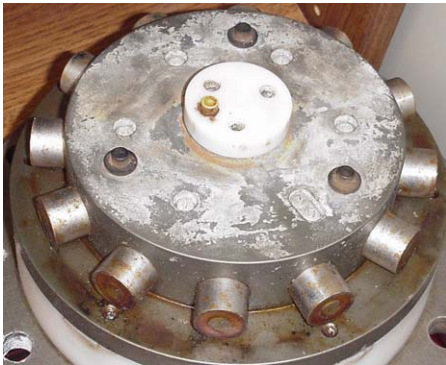
Salt deposits and corrosion resulting from not rinsing surfaces with fresh water
