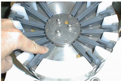
Push trigger to cock release mechanism
