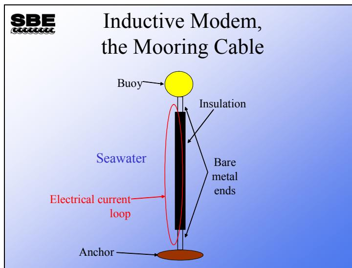
The first current loop is made by the mooring cable itself and seawater. The cable is bare metal on the top and bottom and insulated in the middle.
