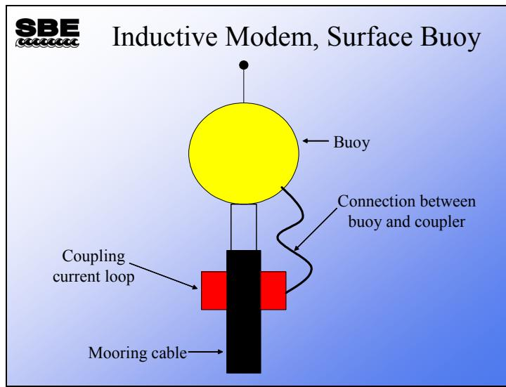
The second current loop is made around the mooring cable. The coupler is a ferrite donut. Ferrite is the stuff that magnetic tape is made from. The electrical current that flows around the coupler induces a current that flows through the mooring cable and the seawater. Thus, the modem signal is transmitted by the surface buoy into its coupler, and the coupler induces a current in the seawater and mooring cable.
