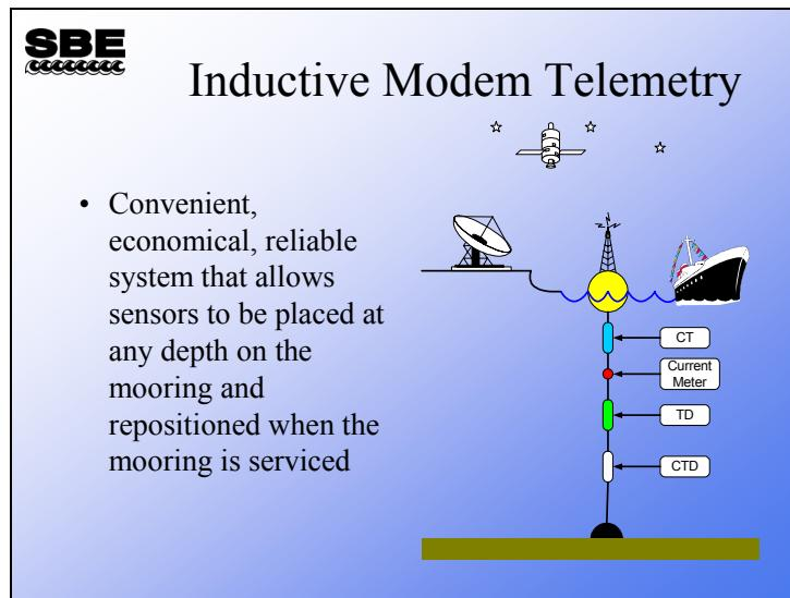
An inductive modem uses electrical current loops to transmit information. Recall from physics class, electrical current flowing in a wire loop induces current to flow in a loop that passes through it. You can think of these loops as links in a chain. The first loop is in the surface buoy. The second loop is formed by the mooring cable and the seawater. The third loop is at the instrument, underwater. Because all coupling is done in loops, no cable breakouts are required.
