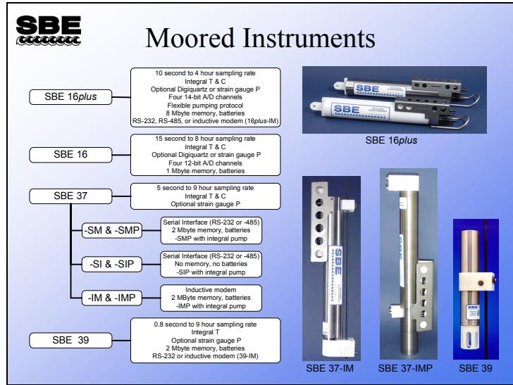
The SBE 16 and 16*plus* are moored versions of the SBE 19 and 19*plus*. The 16*plus* is actually a 19*plus* in moored mode, with optional pressure sensor. The 16 and 16*plus* have the capability to power external sensors and log analog A/D data from them. This is the instrument of choice if you require more data than C, T, and P. The 16*plus* is available with serial interface (RS-232 or RS-485) or inductive modem interface (16*plus*-IM).
