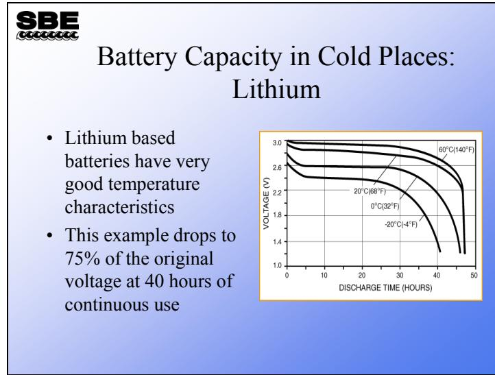
Lithium batteries offer better performance. The main drawback to using them is international shipping restrictions on lithium. For example, the battery pack used by the SBE 37 is made of 6 batteries. It is legal to ship them separately; however, once assembled into the battery pack they become illegal to ship, as they are too large a mass.
