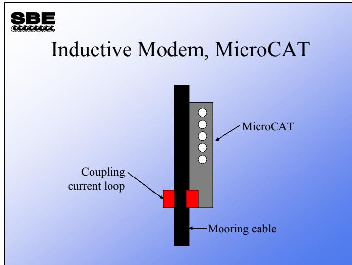
The last loop is at the remote instrument. It has a coupler just like the surface buoy. The current that the surface buoy has induced in the seawater mooring cable loop in turn induces a current in the remote instrument's coupler. The modem in the remote instrument receives and decodes the signal. If the information contained in the signal is addressed to the remote instrument it behaves accordingly, e.g., transmitting a data scan or a status report.
