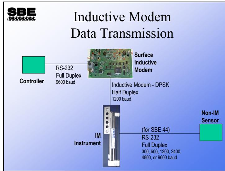
Here are all the players in inductive modem data transmission. The controller is user-supplied and should be able to switch power to the surface inductive modem (SIM). The inductive modem DPSK is via the mooring cable. If you want to use sensors with serial data output made by another manufacturer, the SBE 44 is a stand-alone inductive modem supporting common baud rates with buffering sufficient for most applications.
