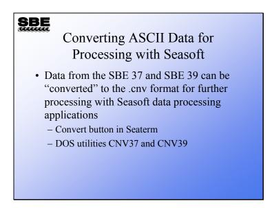
SBE 37s and 39s report data in scientific units in a format that is not compatible with Seasoft's post processing utilities. If you wish to do any processing of this data with SBE Data Processing, you have to convert it to the *.cnv* file format. There is a utility that is part of Seaterm or DOS utilities to perform this conversion.
