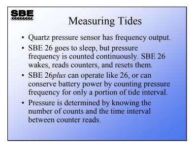
By accumulating pressure sensor frequency counts for the whole sample interval, the SBE 26 / 26*plus* integrates the pressure signal over the entire sampling time. If the sample time is sufficiently long, the influence of surface waves is removed.
