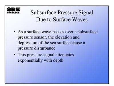
The technique we use to measure tides and waves is to place a pressure sensor underwater and measure the movement of the sea surface above it. One characteristic of this technique is that the signal is attenuated by the water between the sea surface and the pressure sensor. This attenuation can be mathematically modeled and is called the *dispersion relation*.
