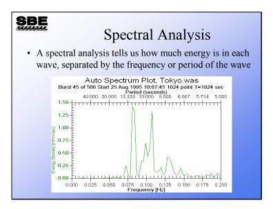
The characteristics of the spectral analysis are determined by the number of data points in the wave burst, the sample rate, and the physical location of the SBE 26 or 26*plus*. The characteristics we are speaking of are the band width or frequency resolution and the maximum frequency of our analysis.
