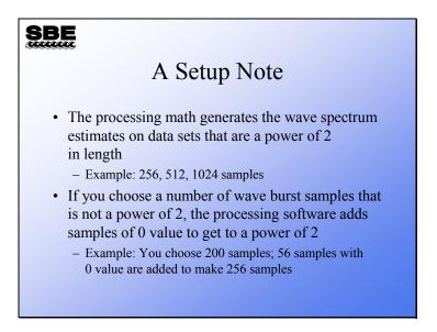
Fast Fourier Transforms are done on data sets that have  $2^N$  elements. If you select a wave burst sample number that is not a power of 2, your data set will be extended to a power of 2 and padded with zeros. While you may save memory this way, you will lose resolution and degrade the statistical confidence you can have in your measurement.
