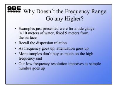
In summary, more samples equals better resolution and better statistics. Your maximum frequency is determined solely by the distance from the sea surface to your instrument and its height off the bottom.
