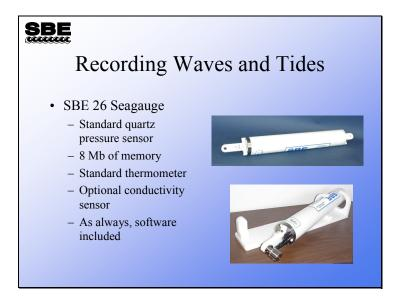
The SBE 26 has been in the field since 1989, and over 400 of these instruments were manufactured. The SBE 26 uses the same pressure sensor as the *9plus*, but the pressure range is much smaller to provide higher resolution. A temperature sensor is standard equipment, and an SBE 4 conductivity sensor may be added as an option.
