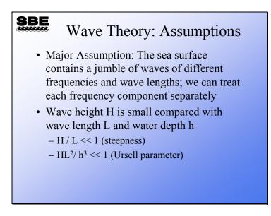
The *major assumption* above is known as linear theory. It supposes that the sea surface we observe is made up of waves of different frequencies, that these waves are superimposed upon one another, and that we can treat each frequency component or wave separately.
