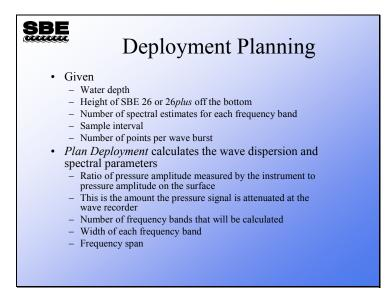
This is the first step. *Plan Deployment* tells you the minimum wave period you can detect given the water depth and the height of the SBE 26 or 26*plus* off the bottom. If you know what period of waves you are interested in, you can adjust your instrument placement to successfully measure these. Conversely, if you have no choice in your instrument placement, you can tell ahead of time what the minimum period wave is that you can measure.
