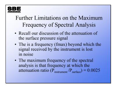
The maximum frequency that we can resolve with our FFT is more severely limited by the attenuation of the pressure signal than by the sampling theory.
