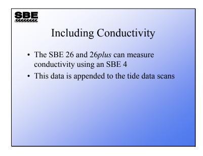
If integrating a conductivity sensor with the SBE 26 or 26plus:
