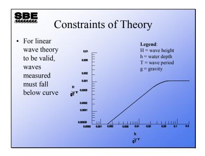
For the math and the test tanks to work out, the waves we can measure with this technique must fall below the line in the plot. Therefore, we are constrained in what sort of waves we can measure.
