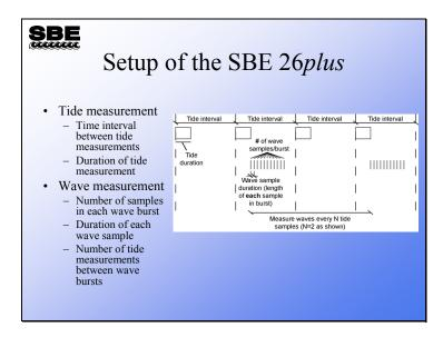
This is just a schematic to illustrate the setup parameters for the SBE 26*plus*. The actual sequencing of the measurements varies, depending on the relationships between the setup parameters.
