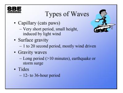
The SBE 26 and 26*plus* are engineered to measure surface gravity waves and tides. Tides are actually waves with very long periods. These two phenomena are those of most interest to scientists and engineers.
