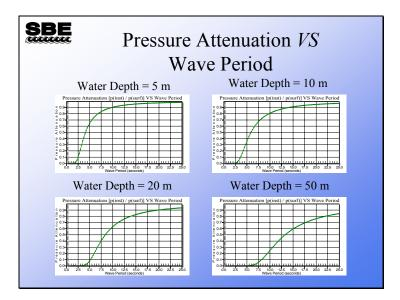
Here are examples of attenuation curves for an SBE 26 or 26*plus* deployed 1 meter off the bottom at 4 different water depths. You can observe that the slope of the curve becomes shallower and that the minimum measurable wave period increases (frequency decreases) as the water depth increases.
