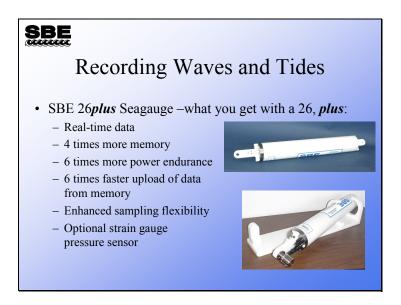
The SBE 26*plus*, an enhancement of the SBE 26, was first manufactured in 2003. While the outside looks the same, and maintains the same dimensions (allowing you to reuse mounting hardware purchased / fabricated for the SBE 26), there are many improvements on the inside. Major improvements / new features are described below:
