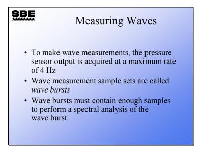
The spectral analysis of wave burst is based on the Fast Fourier Transform. Because of this, the analysis is most accurate if the number of wave burst samples is a power of 2. Further, the more samples in the wave burst, the more accurate the estimation of the wave spectrum. You must balance the desire for accuracy with the endurance of memory and batteries.
