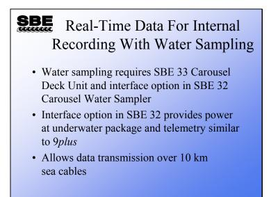
The SBE 19, 19*plus*, and 25 can be equipped with water sampling equipment. The SBE 32 Carousel and SBE 33 Carousel Deck Unit provide power and telemetry for the CTD very similar to the 11*plus/9plus* setup. In addition to water sampling, this equipment allows data telemetry over 10 km of sea cable and supplies more than enough power for the CTD and auxiliary sensors.
