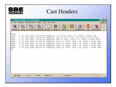
The cast header lists the start date and time, number of scans, number of samples averaged per scan, and reason the cast ended for each cast.
