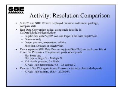
This activity requires some clever use of the processing software. First, use SBE Data Processing's *Data Conversion* module to convert downcast data from C:\Data\Module6\Resolution\Puget25.hex. Then run *Data Conversion* to convert downcast data from C:\Data\Module6\Resolution\Puget19.hex, but skip the first 300 scans; these are invalid data acquired during the instrument package soak.
