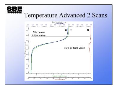
The next step in the process is to advance temperature relative to time to align the temperature and conductivity channels. Note that the salinity spike is much reduced; if the data were bin averaged on 2 decibar bins, the salinity spike would average out of the data.
