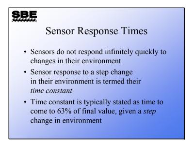
Sensors do not react infinitely quickly to a new environmental condition. For example, let's look at a 2-box ocean, with the top box at 20 °C and the bottom box at 0 °C. If our CTD moved from the top to bottom box, we would see a temperature signal that changed very quickly from 20 °C to 0 °C, but not as a perfectly sharp jump. *The reason for a slower response time for sensors is often found in the packaging of the active element of the sensor*.
