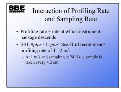
The CTD samples at a fixed rate and the instrument package is lowered through the ocean at a fixed rate. Consider the SBE 9*plus*, sampling at 24 Hz and falling through the ocean at 1 m/s. We would be taking a sample every 4.2 cm.
