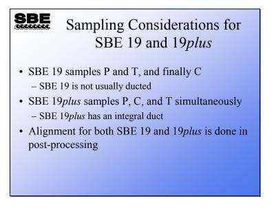
The SBE 19 has a different sampling protocol than the SBE 25 and the *9plus*. The 19 uses the same signal condition circuit, an oscillator, to sample both T and C. A relay switches the oscillator between the thermistor and the conductivity cell. Further, to improve circuit stability, reference resistors are switched into the oscillator every 120 samples.
