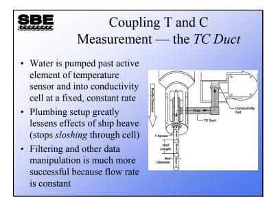
To ensure that the temperature and conductivity measurements are made on a constrained water sample, they are plumbed together and the T-C pair has water drawn through them with a pump that moves water at a consistent, known speed.
