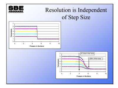
You might think that the resolution of a step change depends on the magnitude of the change. Above are plots of the step response of a filter that closely resembles the temperature response of the SBE 19*plus*. It is obvious that the size of the step does not influence the distance (or time) required to resolve it.
