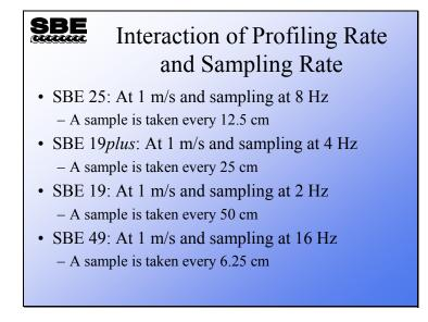
As discussed earlier, the lower sample rates of the SBE 19, 19*plus*, 25, and 49 instruments translates into a coarser resolution than that calculated in the SBE 9*plus* example. The following page illustrates the impact that sample rate has on resolution.
