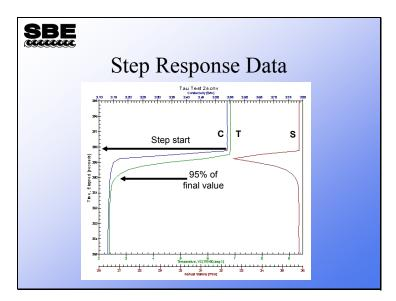
The above plot shows the results of the experiment. The Y axis is time in seconds; this corresponds to decibars at a lowering rate of 1 meter per second. Note that the temperature trace lags the conductivity trace, because the SBE 19*plus* temperature sensor time constant is approximately 0.5 seconds while the conductivity cell has a time constant of about 0.030 seconds.
