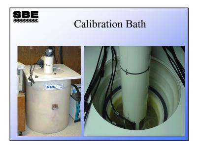
This bath design is common to all of Sea-Bird's calibration activities. The baths are highly insulated and well stirred, and they typically hold temperature to better than  $0.0005~^{\circ}\text{C}$ .
