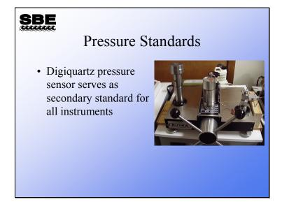
For instruments that have a strain gauge pressure sensor (Druck, Paine, Ametek, etc.), a complete pressure calibration is performed at Sea-Bird, using our Digiquartz pressure sensor as a secondary standard.
