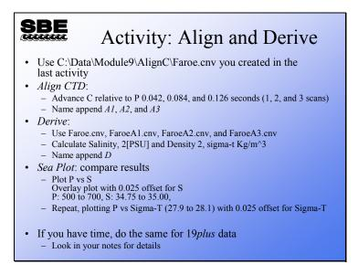
For this activity, start with the .cnv file you created in *Data Conversion* that contains temperature and conductivity. Do some advancing on the file with *Align CTD*. Then, use *Derive* to calculate salinity and density from the original .cnv file and each aligned file. You should end up with the following files:
