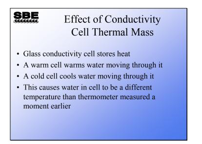
The conductivity measurement has temperature dependence. The conductivity cell itself is constructed of glass and plastic, and as such has a thermal mass. When the cell goes from warm water into cold, the water that passes through the cell is slightly warmed as it transits the cell. Conversely, when the cell comes up from cold water into warmer water, the water that passes through the cell is cooled slightly. This heat transfer can be modeled and corrected.
