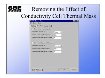
SBE Data Processing has a *Cell Thermal Mass* module. The thermal mass correction is made with the equation shown below, which is a function of amplitude (alpha) and time constant (1 / beta). Like many of the sensor-related phenomena we have considered, the heat transfer within the cell has a time constant.
