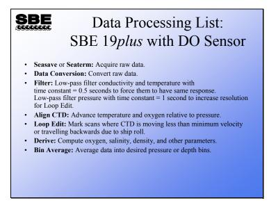
The processing list for the 19*plus* is shorter because of the lower expectations of precision and the different acquisition electronics.
