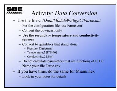
We are preparing to operate on the data with an application that moves the T and C data streams relative to the pressure data stream. Calculation of parameters that are functions of T, C, and P is not useful at this stage. Further, it will complicate and confuse things to have them in the data set before we are ready for them.
