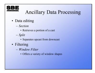
In addition to the data processing modules and procedures we have talked about, there are other modules available. You can clip out part of your data with *Section*, and separate your data into upcasts and downcasts with *Split*. And, there is a window filtering module with various shaped windows.
