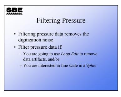
In measuring the pressure sensor signal, there is a digitization error that may be removed by filtering the signal with a low-pass filter. This has the effect of improving the resolution of the pressure signal by smoothing the digitization jitter.
