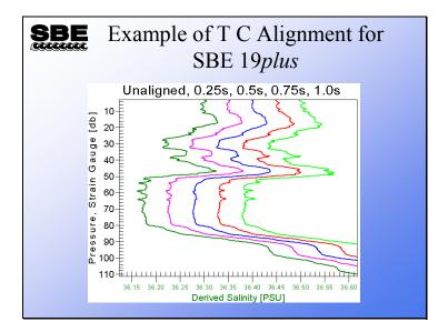
This is from the extra credit data set. The right most trace is the original unaligned data and the others, from left to right, are aligned from 1 to 4 scans. The optimal alignment value may lie between 0.25 and 0.5 seconds; it is left for the reader to experiment and find it.
