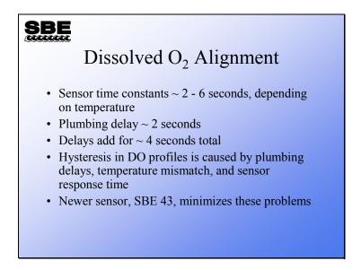
Aligning oxygen current and temperature in relation to pressure can improve hysteresis in dissolved oxygen profiles. The SBE 43 has a faster time constant and shows improvement in hysteresis over the Beckman- or YSI-type of sensor.
