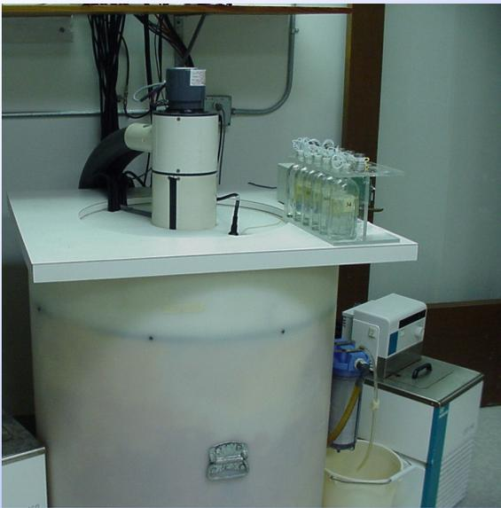
Water sampler on right takes a water sample at every calibration point
