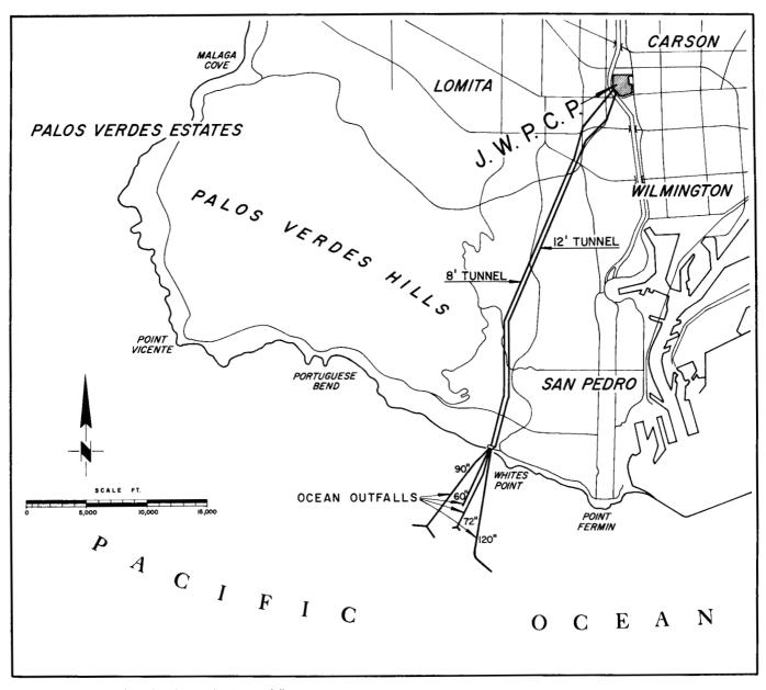
FIGURE 3. Tunnels through Palos Verdes into outfall system.
