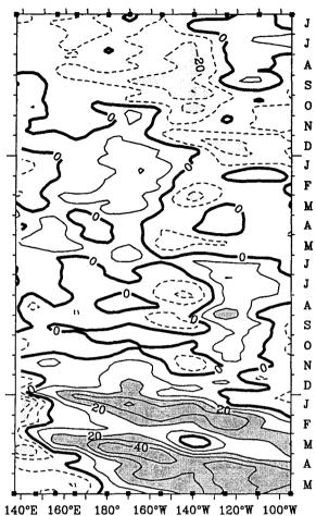
Figure 3. Depth of the 20°C isotherm between 2°N and 2°S for June 1995–May 1997. Analysis based on the five-day averages of moored time series data from the TAO (Tropical Atmosphere Ocean) array. *Shading* denotes isotherm depths more than 20 m deeper than the monthly climatology. Deeper than normal isotherms indicate the eastward propagation of the downwelling phases of two Kelvin waves across the equatorial Pacific in early 1997. Adapted from NCEP (1997b).
