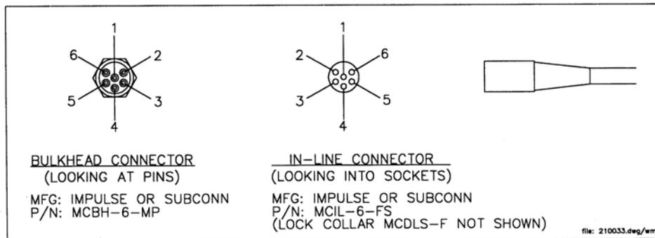
**Figure 7.** 6-pin digital WETStar connector schematic
