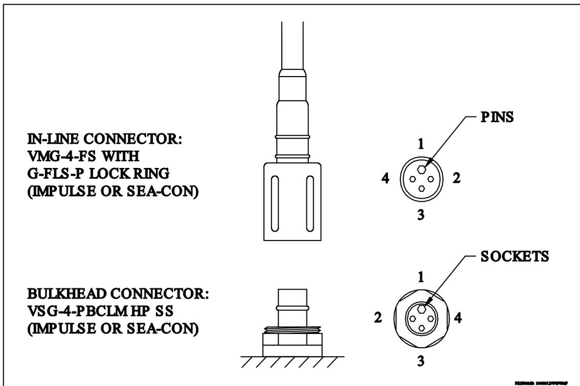
Figure 3. WETStar Bulkhead Connector
