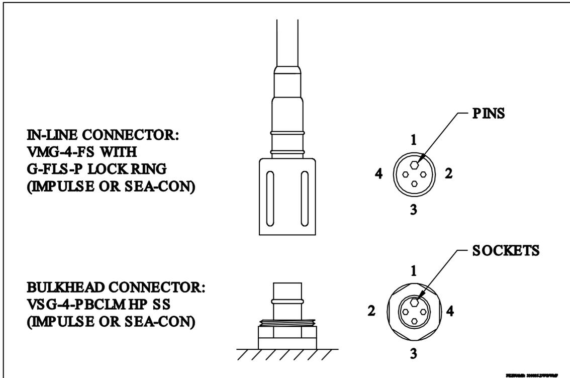
Figure 6. 4-pin digital WETStar connector schematic
