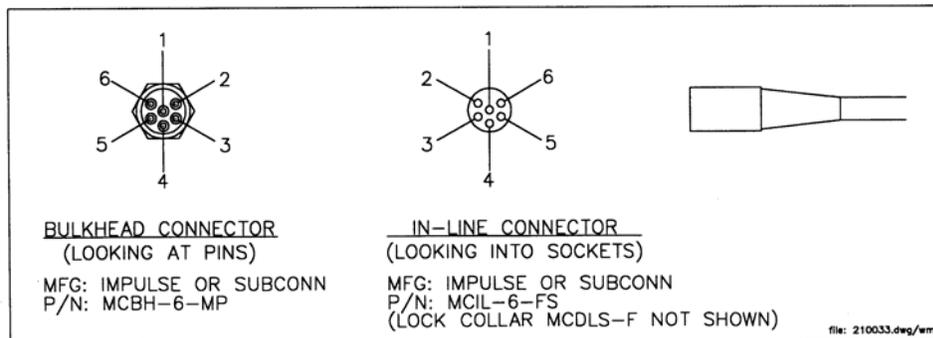
**Figure 7.** 6-pin digital WETStar connector schematic
