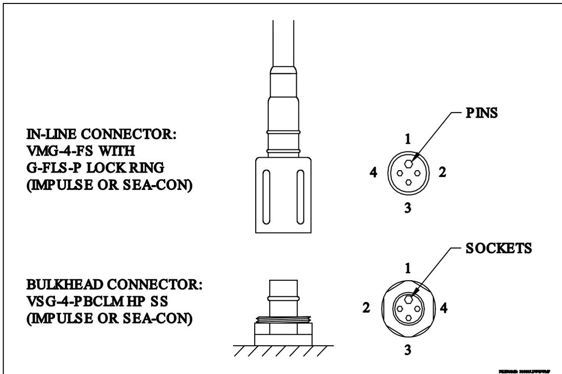
Figure 6. 4-pin digital WETStar connector schematic
