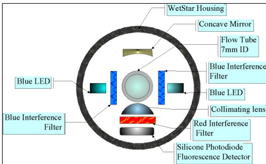
**Figure 2.** WETStar interior components
