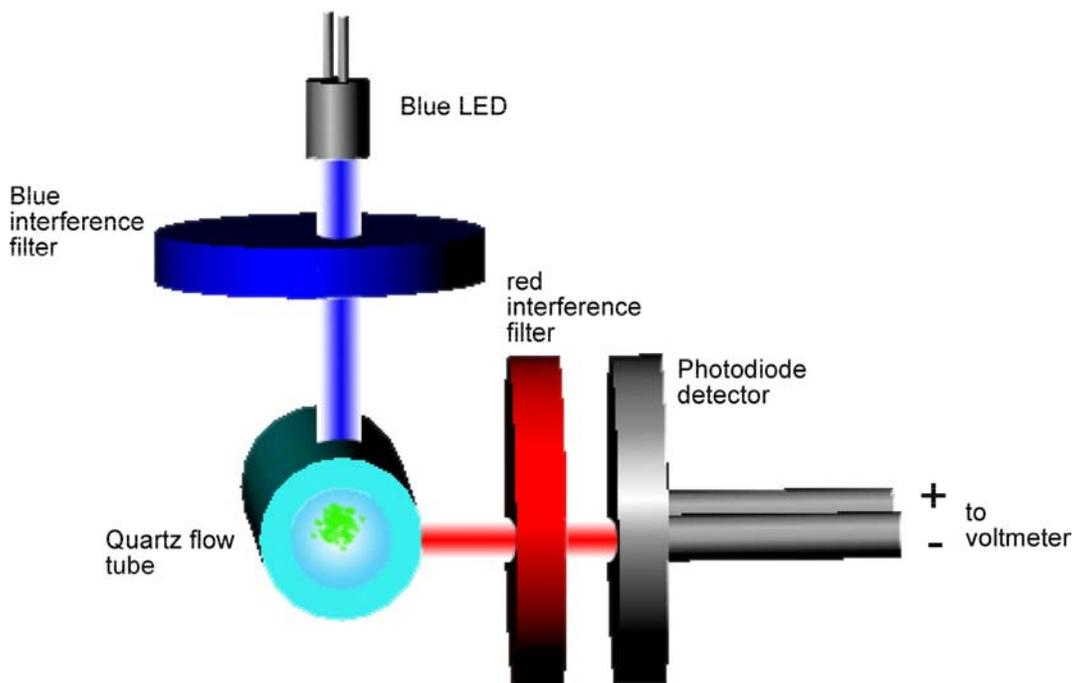
**Figure 1.** Absorption path of blue excitation light
