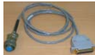
NMEA Interface test cable (Interface Box to NMEA navigation device simulation computer)
