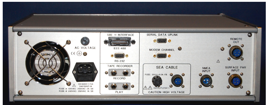
Back Panel – connectors and fuses
