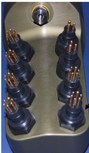
J7 Data I/O, pump, & external power (connects to Y-cable)
