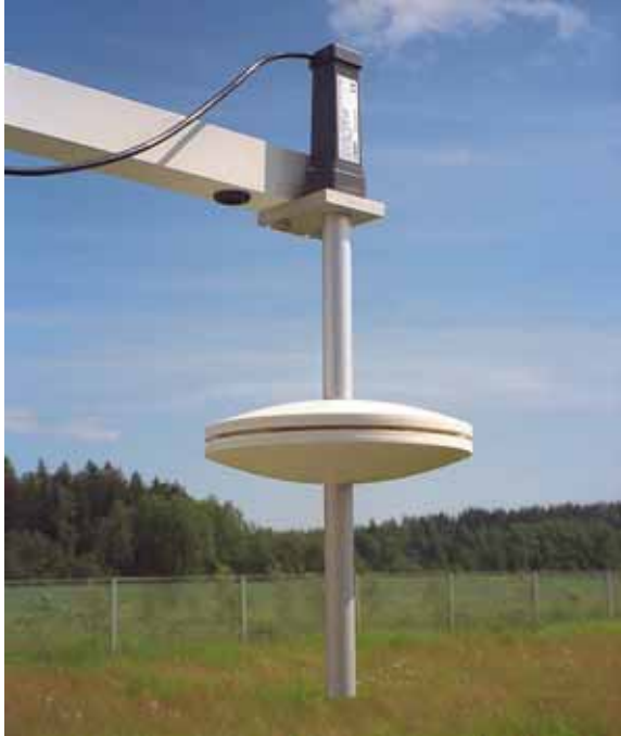
The SPH10/20 is easy to install and connect. In the picture, a SPH10 is connected to a PTB210 barometer.
