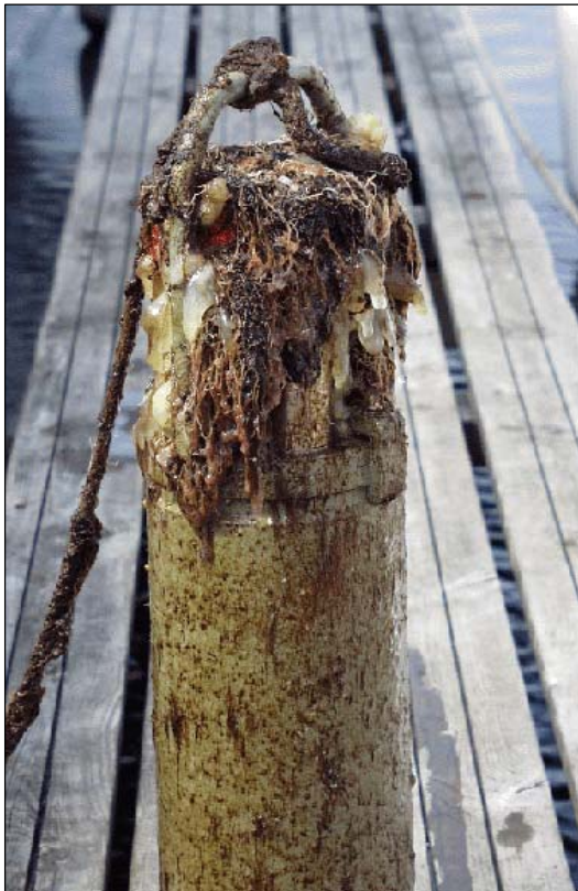
Figure 5-1 Example of fouling on an RCM 9 Mk II with an Oxygen Optode 3830 mounted to it: The Optode was still giving correct readings.
