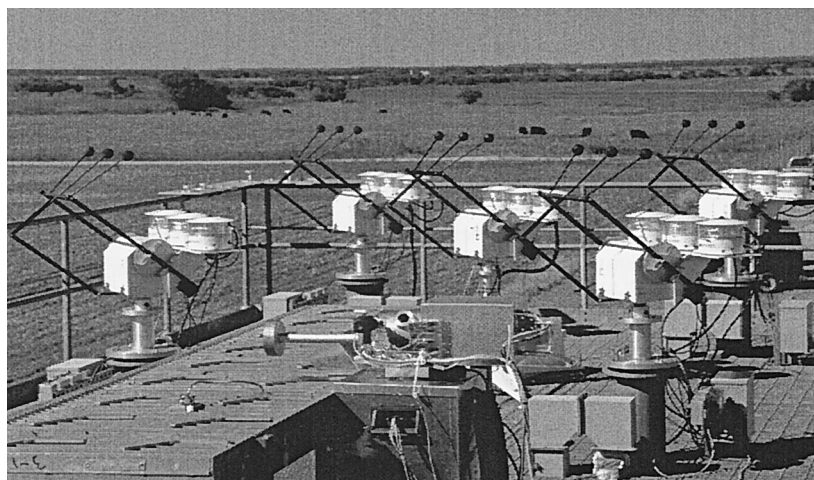
Figure 1. Absolute sky-scanning radiometer and 15 pyrgeometers distributed on five Sun trackers on the roof platform of the SGP radiation trailer.
