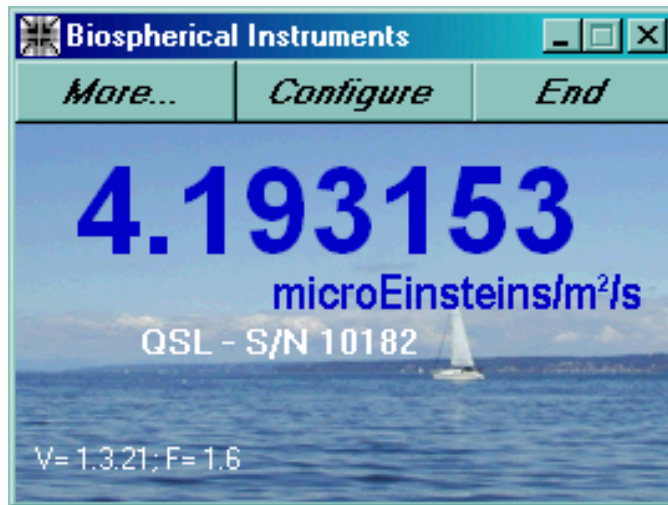
Figure D. Initial data display begins after the software queries the probe for ID and calibration information.
