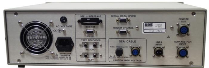
Back Panel – connectors & fuses
