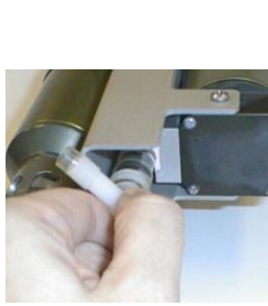
Rotate C Duct clockwise
