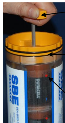
Pull up handle, and unthread cover by rotating counter- clockwise
