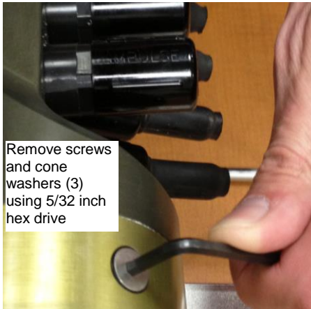
Screw and cone washer
