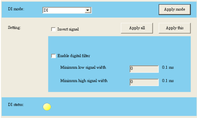
Figure 5.14: Individual Channel Configuration: DI
