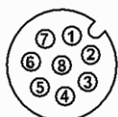
SPN1 analogue output connector pin-out (looking at pins on SPN1)
