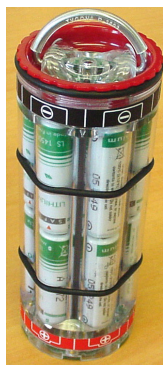
Assembled battery pack
