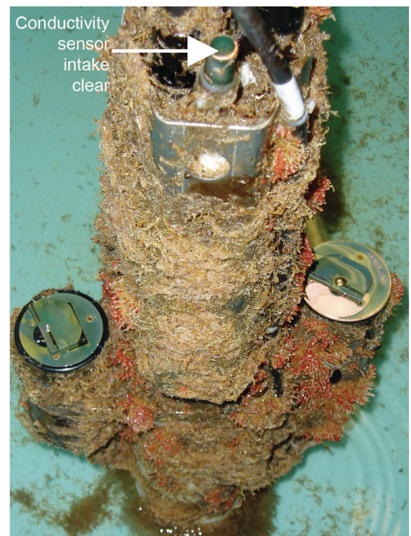
SBE 16plus SeaCAT CTD after recovery. Outside of CTD encrusted, but intake to Conductivity sensor clear, indicating that inside of cell is clear as well.
