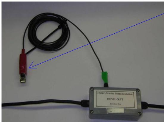
DO NOT connect ship's hull to more than one location
