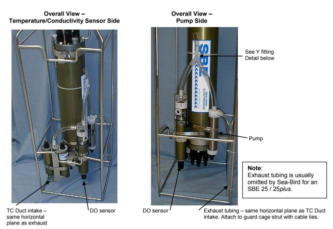
Temperature/Conductivity to DO Sensor Detail
