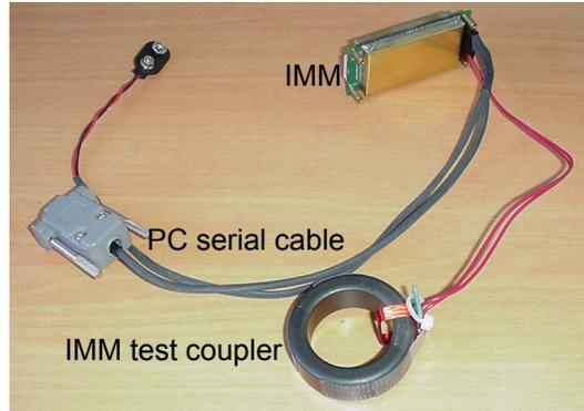
3. Apply power to the SIM and connect it to a different PC serial port. Run SEATERM or another terminal program. If using SEATERM, select Configure/SBE 37, and on the COM Settings tab select RS-232 mode. Select the appropriate COM port at 9600 baud, 8 bits, no parity, 1 stop bit. Select no flow control if using a terminal program other than SEATERM. The terminal program displays an S> prompt when you press Enter.
