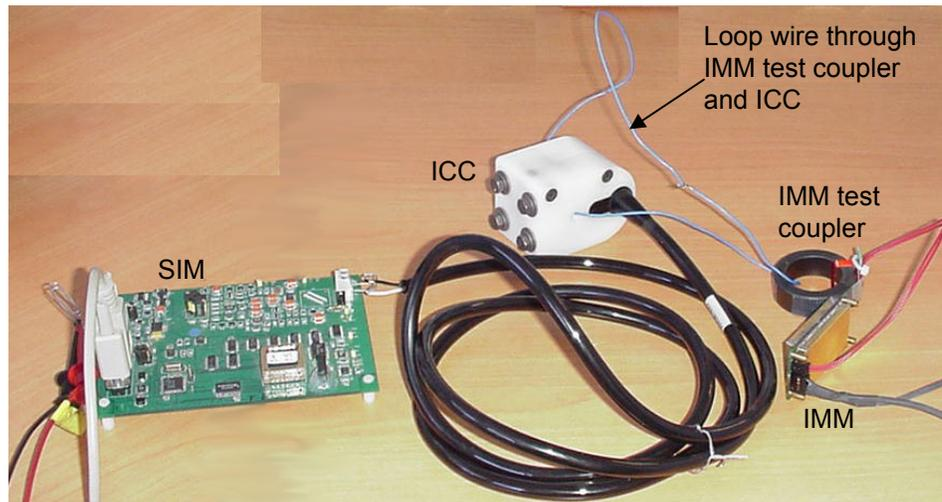
5. Connect a 9-volt battery to the IMM. The terminal program displays an IMM> prompt when you press Enter.
