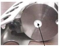
Standard pressure sensor port plug. (*Note*: Photo is SBE 37-SM. Pressure port details are similar for all instruments included in this application note)
