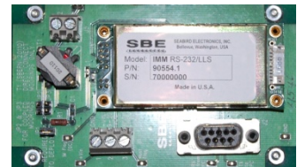
Figure 18: IMM with Direct Connect PCB
