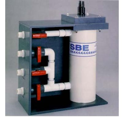
field cell makes possible the use of expendable anti-foulant devices (supplied). The same conductivity cell and stable interface electronics have been used on thousands of SBE 16 / 16 plus (moored) and SBE 19 / 19 plus (profiling) SEACATs in use around the world today.
