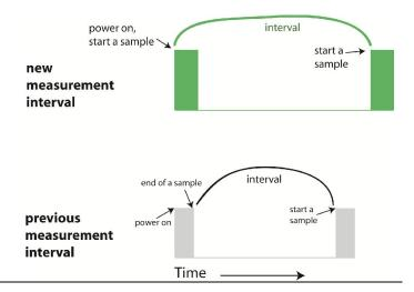
The manufacturer recommends that the user do a test cycle of data collection before a deployment to understand how the Data Rate, the Set Number of Samples, and the Set Cycle Interval function together.
