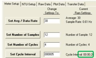
(sample rate, seconds x Data Rate) + entered Interval value +  $\sim$ 3 seconds for wiper = calculated Interval time (1.6 x 12) + 5 + 3 = 27.2  $\sim$  28 seconds, the calculated Interval time.
