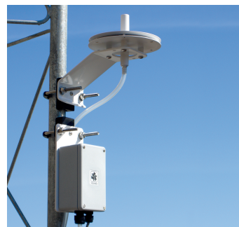
Weatherproof Enclosure and Pressure Port
