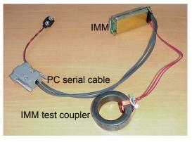
3. Connect a 9-volt battery to the PC Serial cable. The terminal program displays an IMM> prompt when you press Enter.
