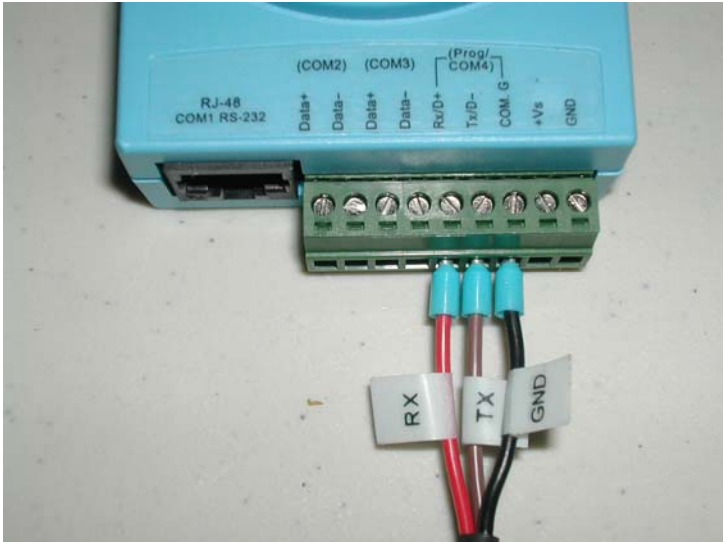
Figure 2-10 Cable Configuration Wiring
