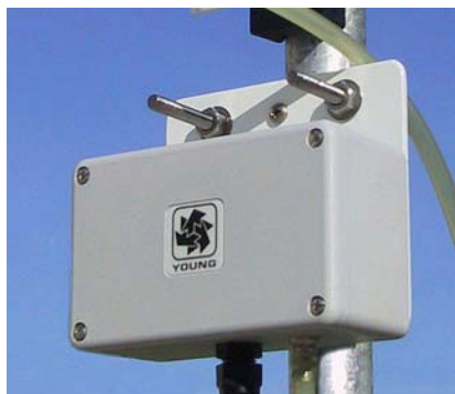
61202 Barometer mounted on mast.
