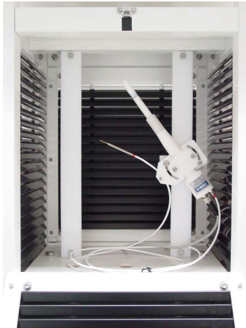
Figure 5 HMP155 with T-Probe Installed in Stevenson Screen
