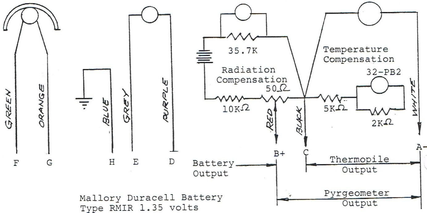
Fig. 4. Schematic for elimination the effect of detector temperature on the measurement of infrared radiation fluxes (including temperature compensation circuit and connections for checking thermopile and battery outputs)
