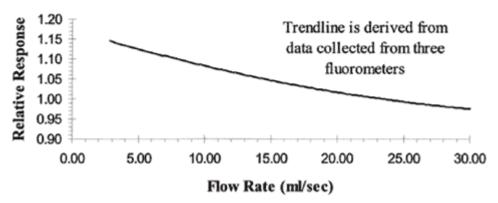
It is possible to use the sensor in a profiling mode without a pump. However, it is difficult to keep a constant flow rate through a sensor cage because of sea-states and ship motion.
