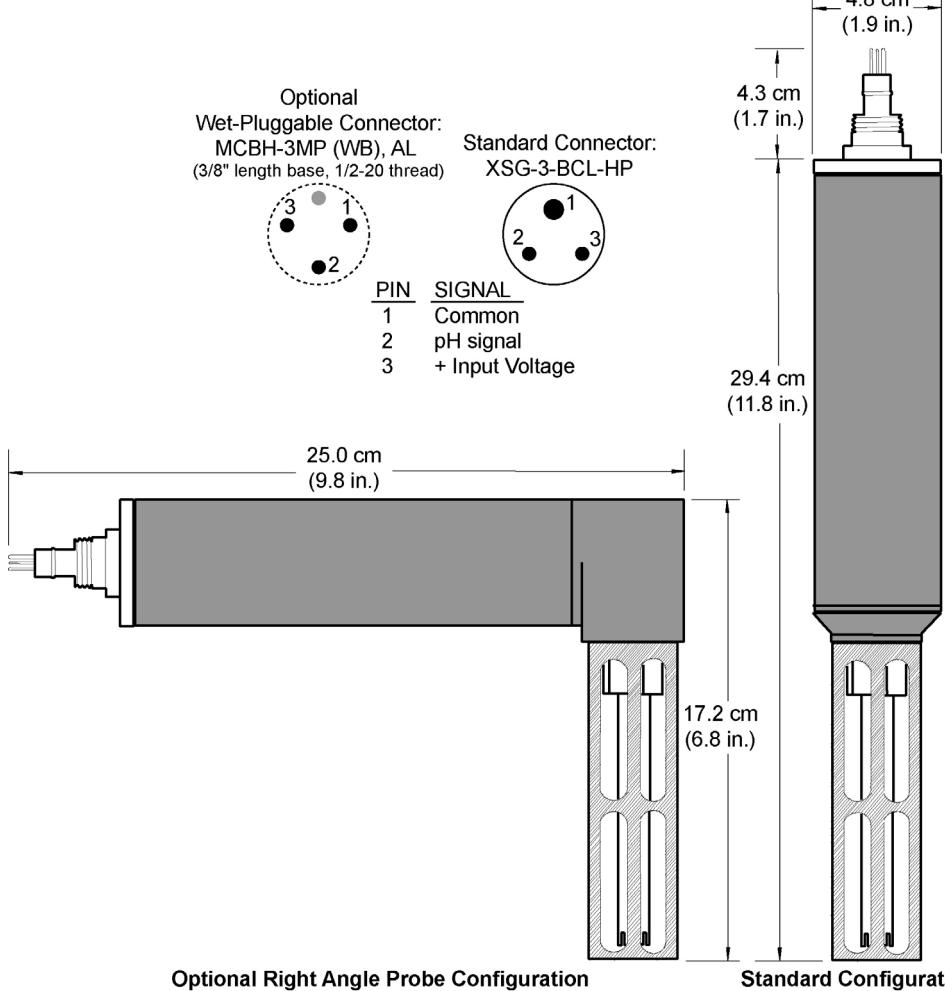
**Note:** SBE 18 must always be mounted with the pH probe in a vertical orientation, as shown in drawings at left. A right angle probe configuration is typically required for applications where the CTD is mounted horizontally (for example, in an extension stand below an SBE 32 Carousel Water Sampler), and the SBE 18 is mounted to the CTD.
